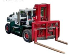
As our crane hire and transport business continue to expand, offering forklift services has become a no brainer due to its vital function in lifting unusual loads. They can assist in the mobility of machinery. Forklifts are an economical way of moving cargo off trucks with metal forks installed at the front of the vehicle for lifting.
