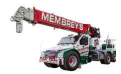
The AT40 offers the latest in pick + carry engineering and technology. Boasting a 44% larger load capacity than the MAC 25, the mighty AT40 pick and carry crane has a maximum lifting capacity of 40 tonne. The articulated 3-axle design of the AT40 gives it a similar turning circle to the MAC 25.
