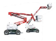
Both articulating boom lifts and telescopic boom lifts can tackle tough jobs. A telescopic boom lets you reach farther with more capacity, putting you right where you need to be as simply and efficiently as possible. But, if the job requires you to get up and over objects, an articulating boom lift offers greater flexibility.
