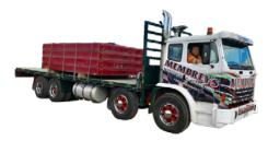
Tray trucks are small to medium-sized trucks often with drop side rails for loading ease. These are generally used in business delivery projects, warehousing, steel transportation and transportation of structural items. These trucks have a carrying capacity that ranges from 1.7 to 9 tonnes and are up to 7 metres in length.
